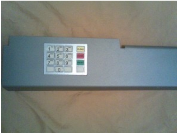
A bogus PIN pad overlay
