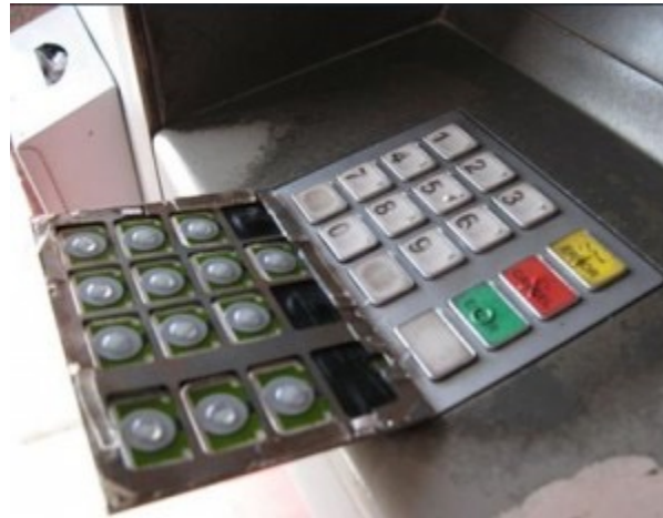
ATM PIN capture overlay device pulled back to reveal legitimate PIN entry pad
