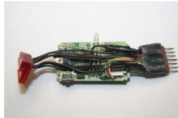
Bluetooth-enabled gas pump skimmer
